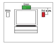
The center channel speaker should be placed slightly behind the front left and right speakers, and no more than two feet above or below the tweeters of the left and right speakers. It is often convenient to set the center speaker on top of the television set, as shown in the drawing.
